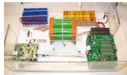
Figure 2 Electric vehicles and UPS applications might use various battery types, all of which need monitoring with battery-stack-measurement ICs (courtesy Linear Technology).
